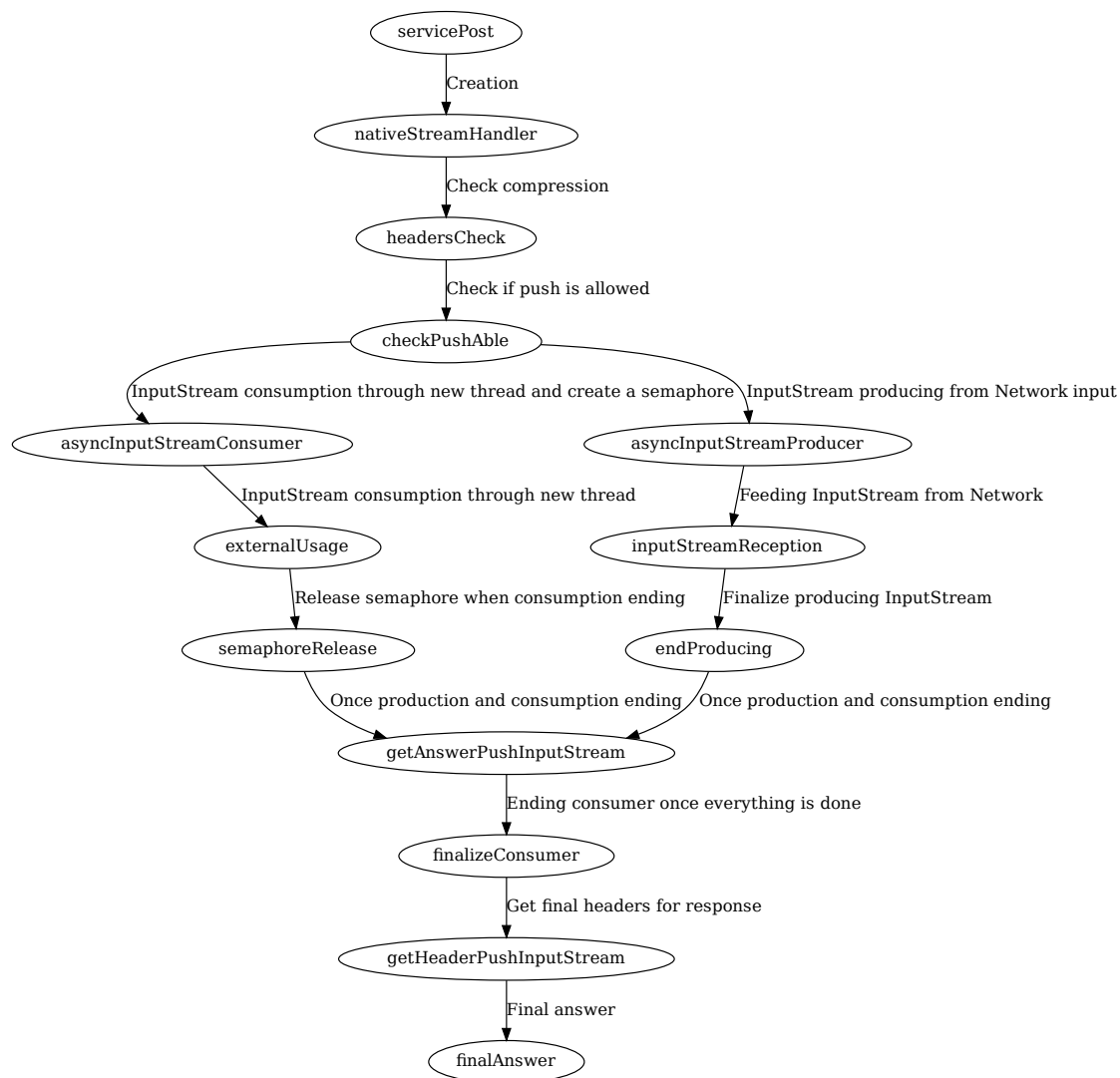
Fig. 2: Illustration of network steps in receiving InputStream within server
